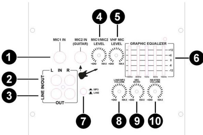
1. Input connector for microphone.
