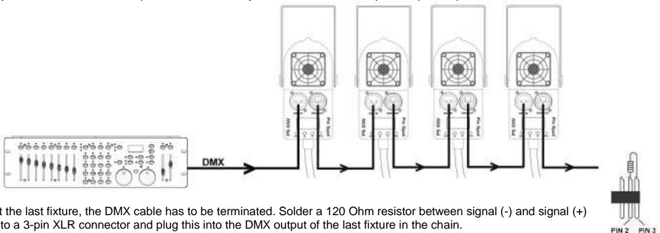
At the last fixture, the DMX cable has to be terminated. Solder a 120 Ohm resistor between signal (-) and signal (+) into a 3-pin XLR connector and plug this into the DMX output of the last fixture in the chain.
