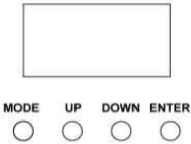
The control board offer several features: you can simple set the starting address, run the pre-programmed program or make a reset. The main menu is accessed by pressing the **Mode**-button, browse through the submenu by pressing **Up** or **Down**.
